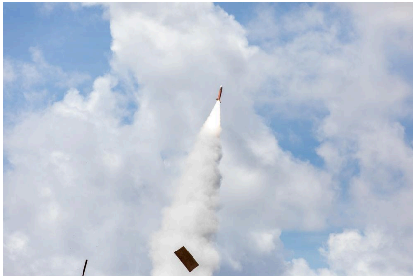
Figure 4. A PAC-2 Patriot interceptor launches during a 2022 live-fire exercise in Palau. The engagement used external F-35 sensor data, illustrating that missile defence is a network rather than a stand-alone launcher. U.S. Army photo; public domain. 16
