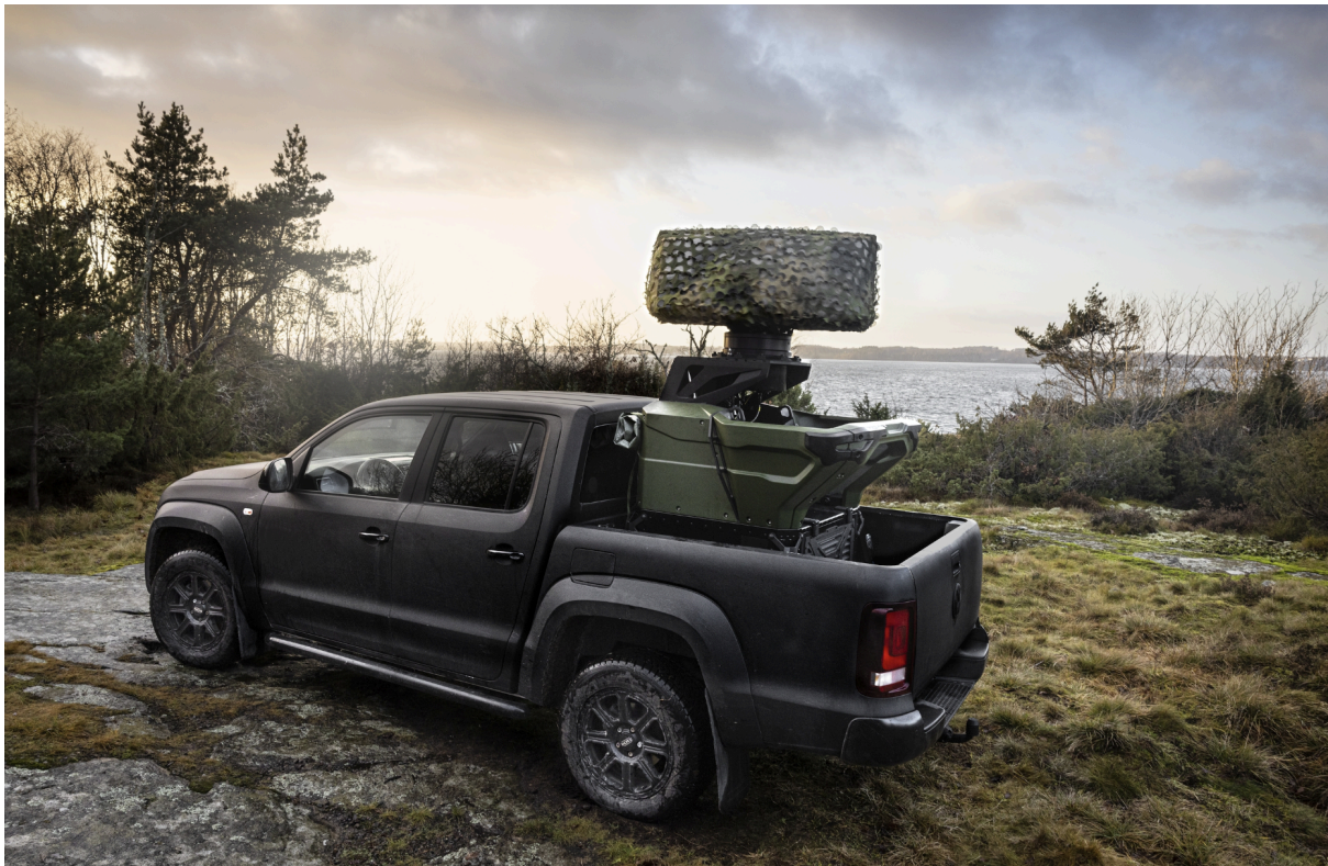
Source: Saab. Giraffe 1X on pickup - Distributed, mobile short-range radar.
