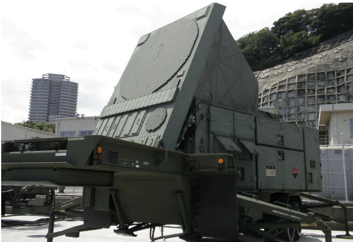
Source: Missile defense advocacy alliance. Patriot AN/MPQ-53/65 radar - a large, high-value air-defence radar system designed for traditional air and missile defence
